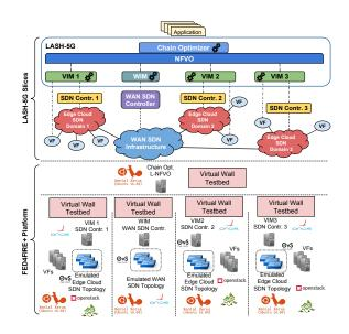
Fig. 1. Reference architecture and LASH-5G deployment on Fed4FIRE+.
