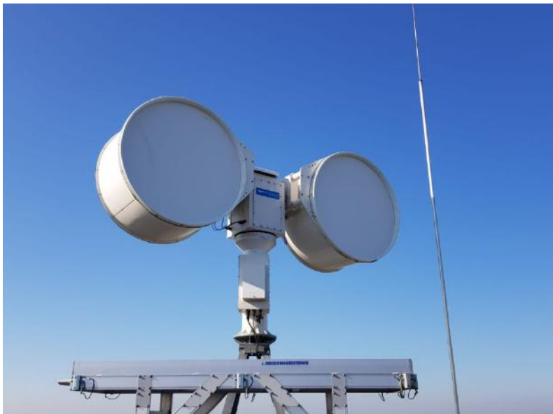
X-band weather-radar hardware, deployed at 153m tall building in Rotterdam, Netherlands
