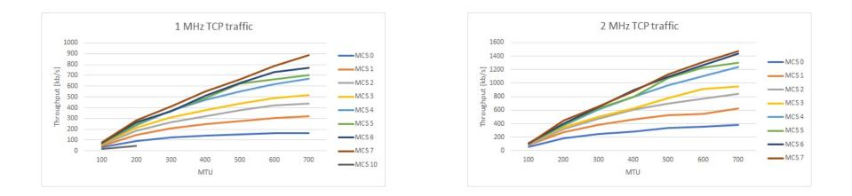
Default parameters: TCP traffic, Normal Acknowledgement, No aggregation, Long Guard interval, 1x1 Spatial stream
